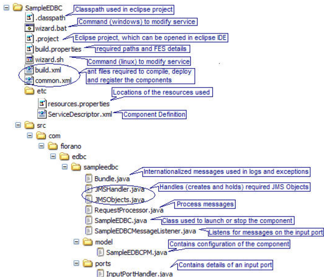
Figure 3.6.31: Structure of asynchronous component
