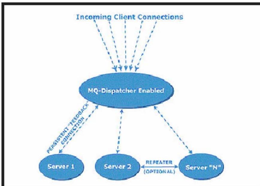
The dispatcher component of FioranoMQ Server is typically connected to multiple FioranoMQ servers, which can run on different machines or on the same machine. All of these servers become part of the "cluster" that is serviced by the dispatcher.
