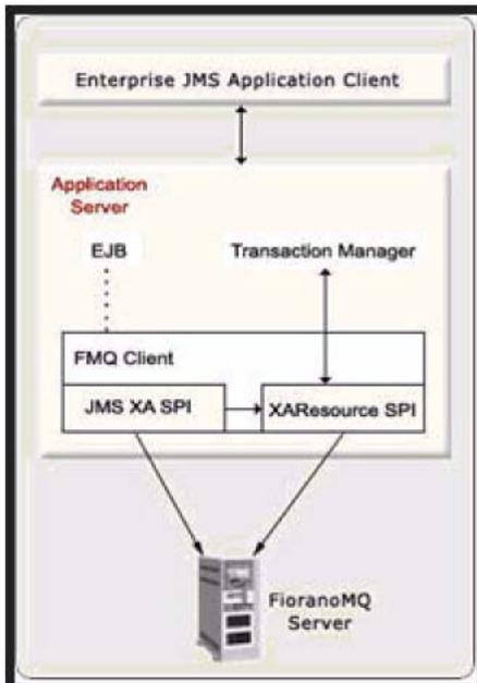
The application logic is required to be written at a much higher level, without regard for the specific underlying transaction system. The low-level transaction system is totally abstracted by the EJB container that runs behind the scenes.
