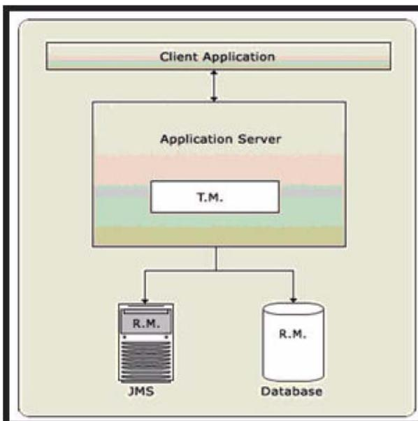
A transaction manager provides the services and management functions required to support transaction demarcation, transactional resource management, synchronization, and transaction context propagation.
