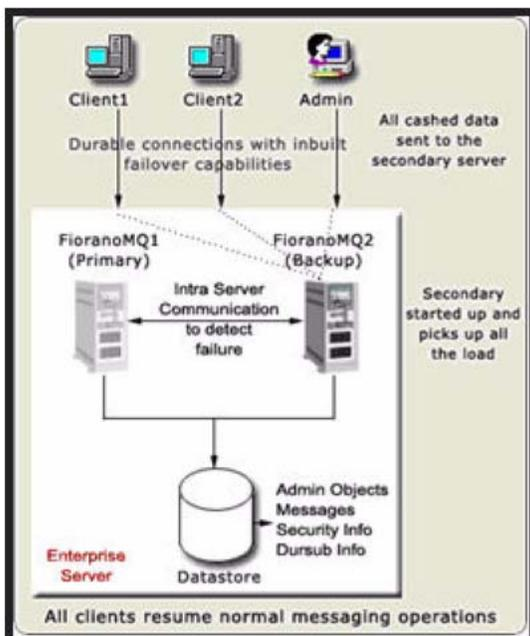
Upon restarting the primary server, it would detect that its backup is alive and enter into passive mode. It would continuously ping the backup server and initiates its startup sequence if the backup server goes down due to any reason.
