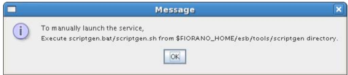
Figure 7: Pop up window showing the steps for launching the component instance manually
