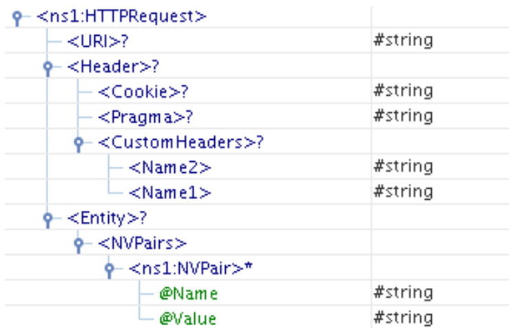
Figure 14: Schema when custom headers are selected
