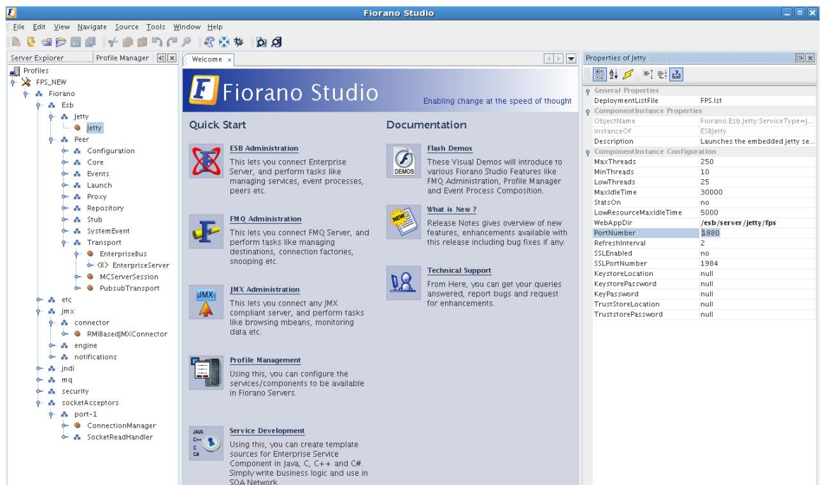
Figure 2.4.15: Changing Jetty port
