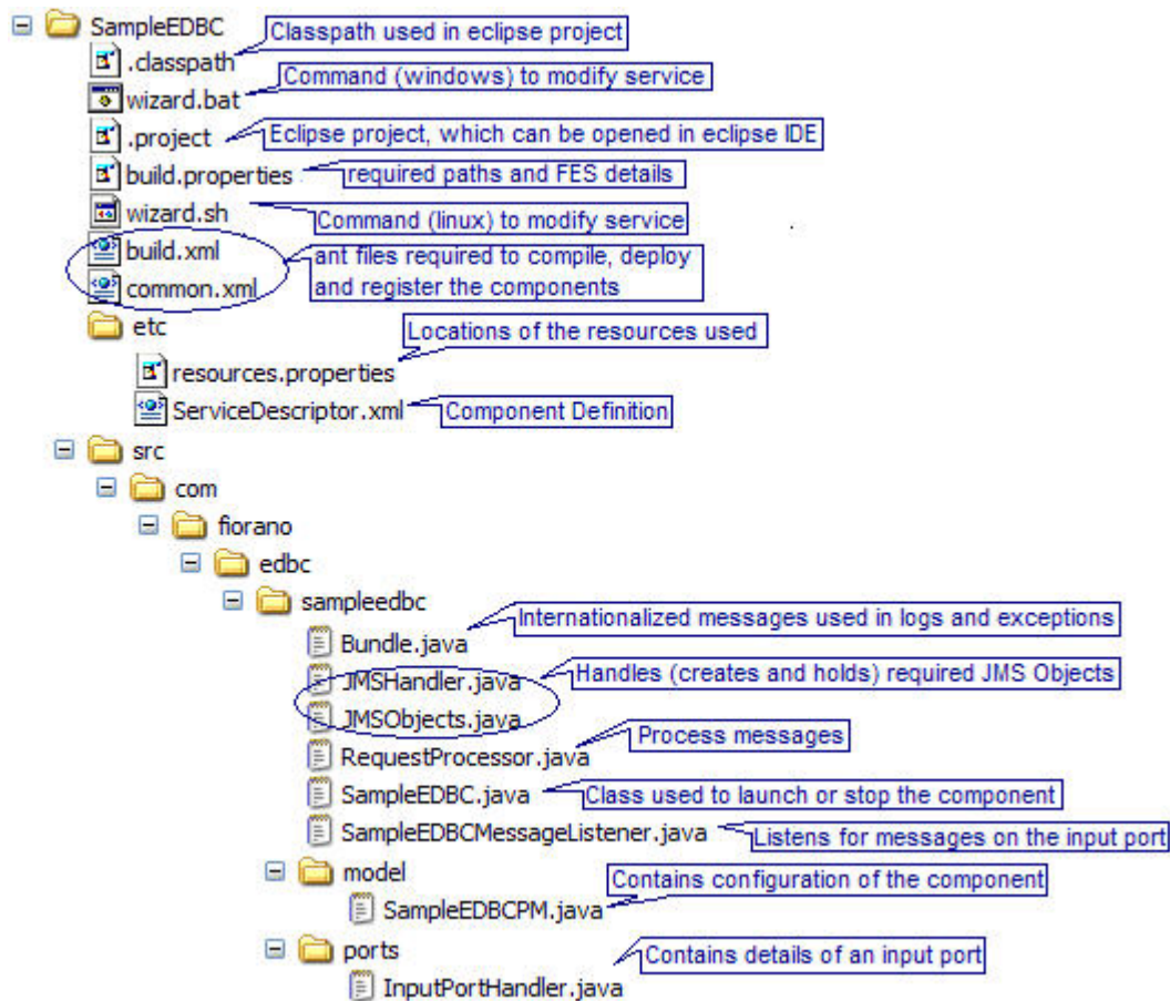
Figure 3.6.31: Structure of asynchronous component
