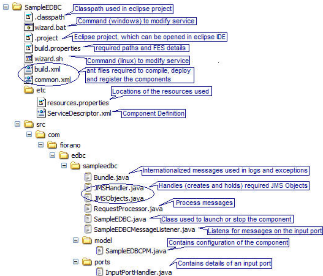
Figure 3.6.31: Structure of asynchronous component
