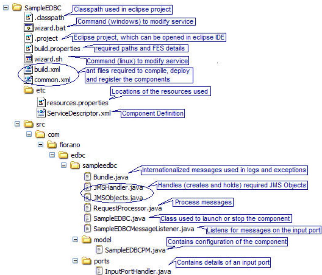
Figure 3.6.31: Structure of asynchronous component
