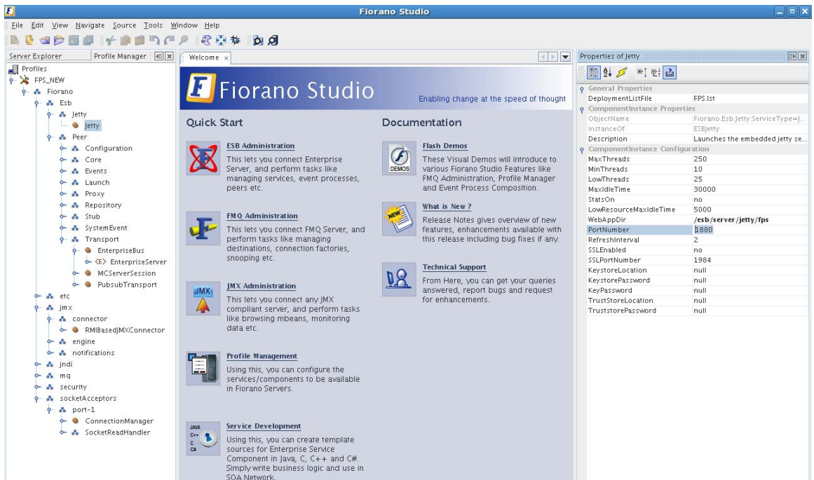
Figure 2.4.15: Changing Jetty port
