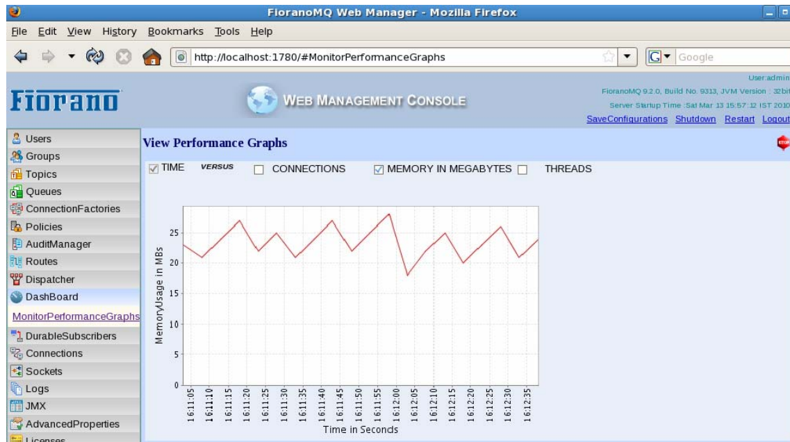
Figure 32.19: Displaying a graph of Time Vs Memory
